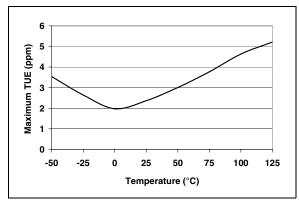
FIGURE 2-22: Maximum TUE vs. Temperature.
