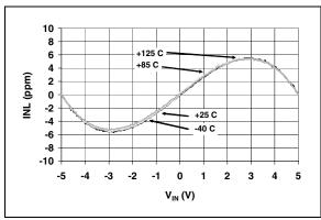
**FIGURE 2-3:** INL Error vs. Input Voltage  $(V_{DD} = 5.0V, V_{REF} = 5V).$
