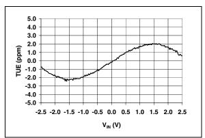
**FIGURE 2-18:** Total Unadjusted Error (TUE) vs. Input Voltage ( $V_{DD} = 2.7V$ ).
