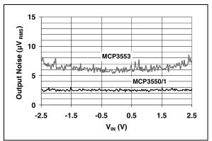
FIGURE 2-7: Output Noise vs. Input Voltage ( $V_{DD} = 5.0V$ ).
