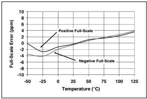
FIGURE 2-14: Full-Scale Error vs. Temperature.
