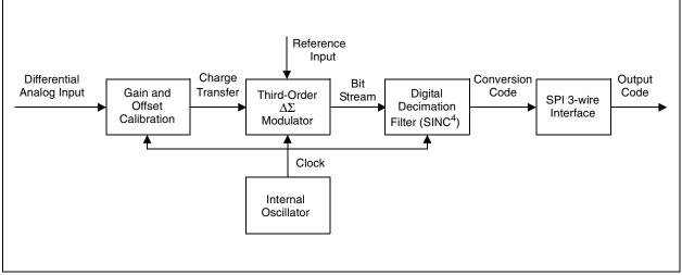
FIGURE 4-1: MCP3550/1/3 Functional Block Diagram.
