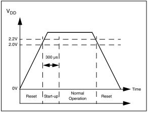
FIGURE 4-6: Power-On Reset Operation.
