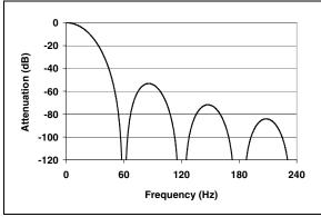
FIGURE 4-3: SINC Filter Response, MCP3550-60 Device.
