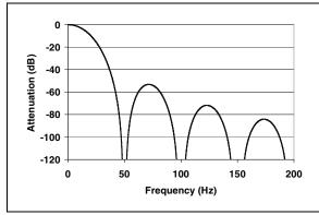
FIGURE 4-2: SINC Filter Response, MCP3550-50 Device.
