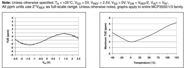
FIGURE 2-19: Total Unadjusted Error (TUE) vs. Input Voltage.
