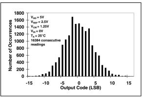
FIGURE 2-17: MCP3553 Output Noise Histogram.
