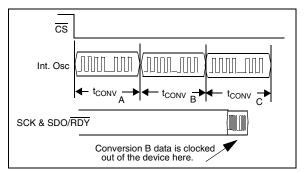
FIGURE 5-5: Most Current Continuous Conversion Mode Data.
