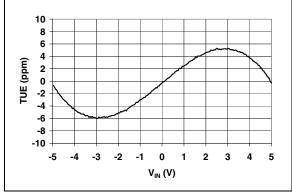
FIGURE 2-20: Total Unadjusted Error (TUE) vs. Input Voltage (V<sub>REF</sub> = 5.0V).
