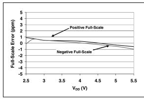
FIGURE 2-13: Full-Scale Error vs. V<sub>DD</sub>.
