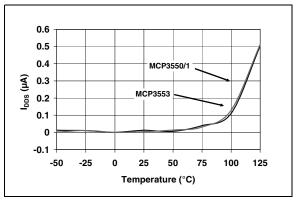
FIGURE 2-24: I<sub>DDS</sub> vs. Temperature.
