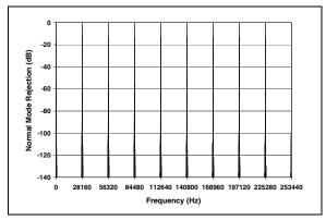
**FIGURE 4-5:** SINC Filter Response at Integer Multiples of the Sampling Frequency (f<sub>s</sub>).
