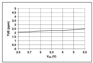
FIGURE 2-23: Maximum TUE vs. V<sub>DD</sub>.
