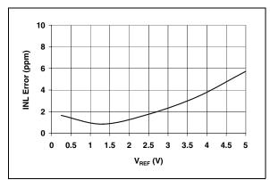
FIGURE 2-4: Maximum INL Error vs. V<sub>REF</sub>.
