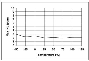
FIGURE 2-5: Maximum INL Error vs. Temperature.
